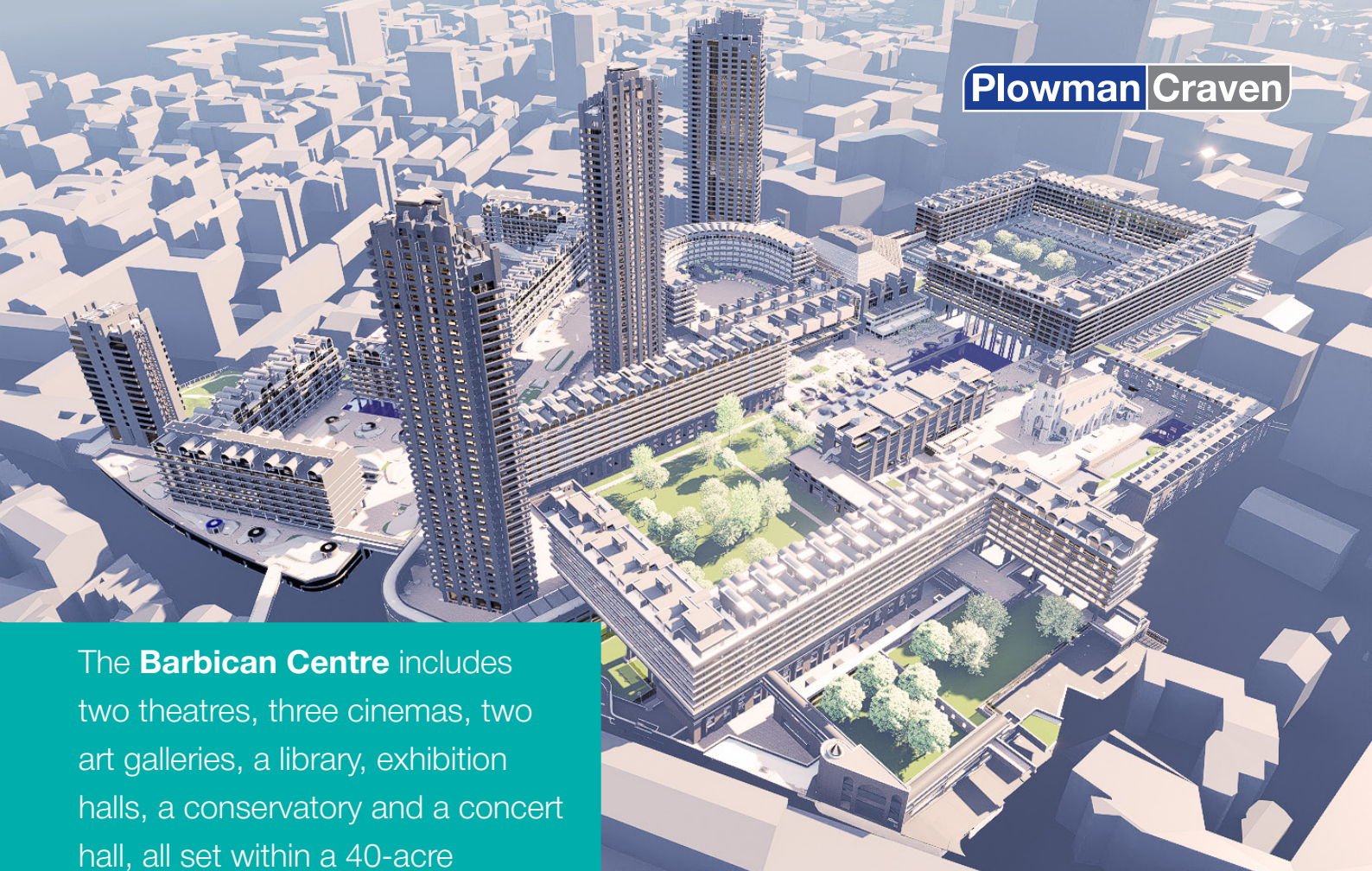
BIM model of the entire Barbican estate, including full LOD3 model of the Arts & Conference Centre
