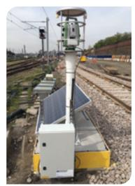
parameters were met and a system encompassing track prisms mounted along both running rails was installed allowing core parameters of cant, twist and displacement to be recorded. This was supplemented by structural prisms on retaining walls adjacent to a canal.
